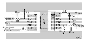
Figure 3. PCB Layout Guide
