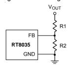
Figure 1. Setting Output Voltage
